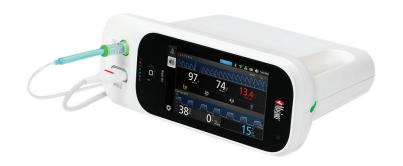
The Rad-97 CO2 monitor and pulse oximeter features Signal Extraction Technology (SET®), Measure-through motion and low perfusion pulse oximetry with rainbow SET technology. Masimo SET® demonstrates thee highest sensitivity and specificity in identifying desaturation events during conditions of motion and low perfusion.
