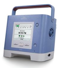
Using a new single limb circuit and proximal flow sensor, Trilogy 200 offers improved triggering and leak compensation that allows for the more sensitive delivery of therapy. This added sensitivity decreases work of breathing, resulting in greater comfort, better ventilation, and improved patient/ventilator synchrony for a wide range of adult and pediatric patients.
